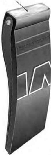
3. **Use a sponge and a paste-type lubricant to lubricate the tire bead sole according to the photo shown to the left.**
