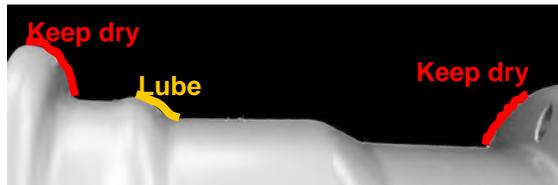
4. **If more than 40 psi is required to seat the beads, dismount the tire, re-lubricate and repeat the process. Always follow the advice of the tire and wheel manufacturer regarding maximum pressure.**
