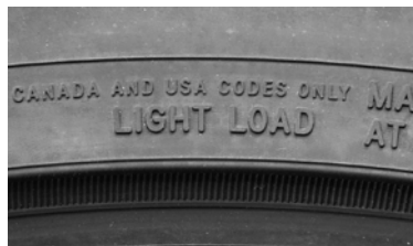
Figure 1 - Light Load molded into sidewall
